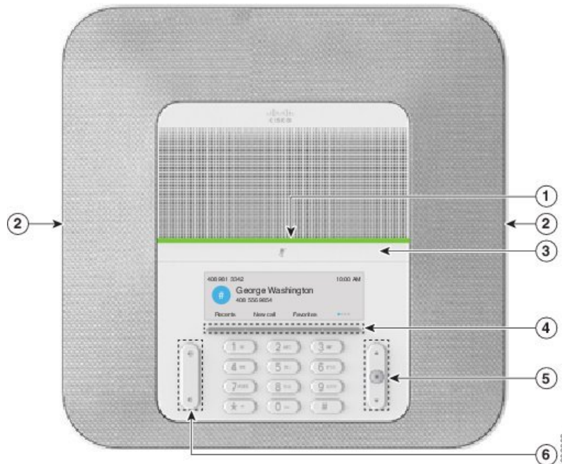
Figure 11: Cisco IP Conference Phone 8832 Buttons and Features
